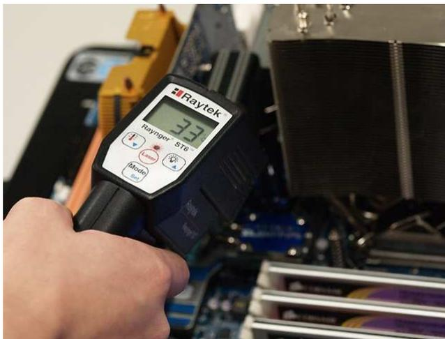
Running the stress program, the temperature of North Bridge is 33°C
