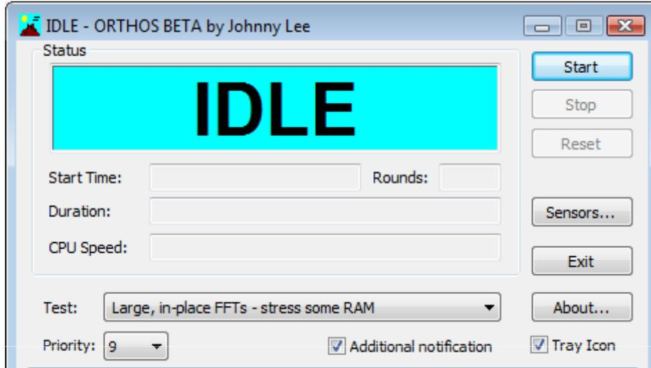
Next open 4 SP2004 programs (burn-in tool used to fully load the CPU), set Large, in-place FFTs and priority to 9. This mode will stress the maximum heat of the processor, and will quickly determine if the CPU is stable or not. Next open the task manager. Because SP2004 only supports 2 threads (the i7 920 has 8 threads in total), you need to run 4 SP2004 programs and assign 2 cores (threads) to each SP2004.
