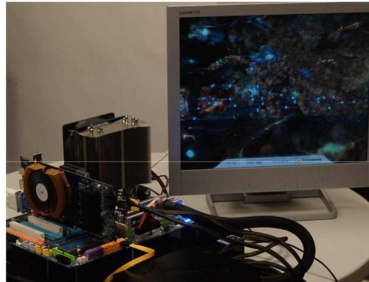
Successfully passing the test, 4GHz seems to be stable. Regarding the performance improvement, from our default score of 17465 we have now reached 23931, a 37% improvement (4GHz VS. 2.83GHz with Turbo boost default enabled).
